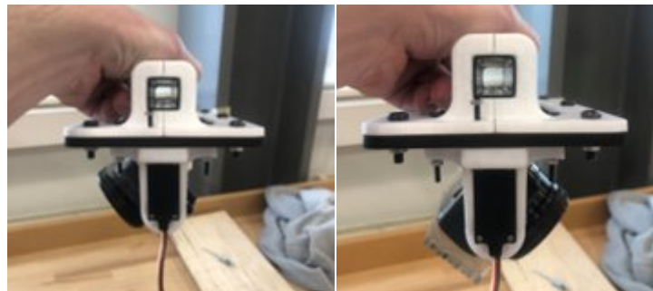
Figure 32 - Pictures of gimbal at maximum deflection during timing test
