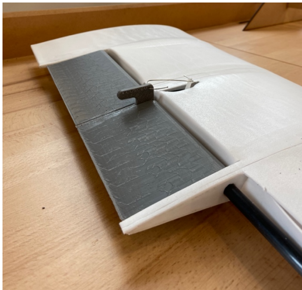
Figure 26 - Final control surface design showing fully integrated control horn
